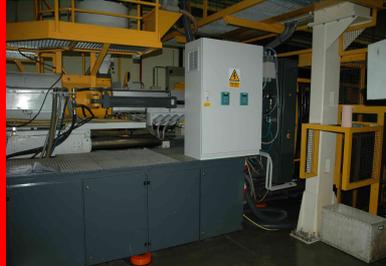
two-motor SyncroSpeed enclosure mounted on Engel ES4400/500
