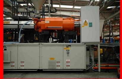
single 90kW SyncroSpeed enclosure mounted on Engel ES4550/600
