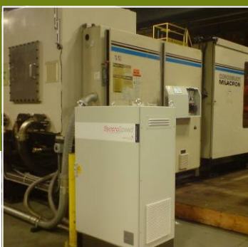
Wisconsin, USA SyncroSpeed 135 HP 2-motor system installed on a Cincinnati 725t
